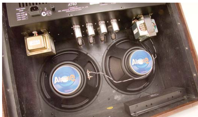
The vast expanse of the Akita's cabinet houses two 12" speakers and a mini Accutronics reverb tank.
